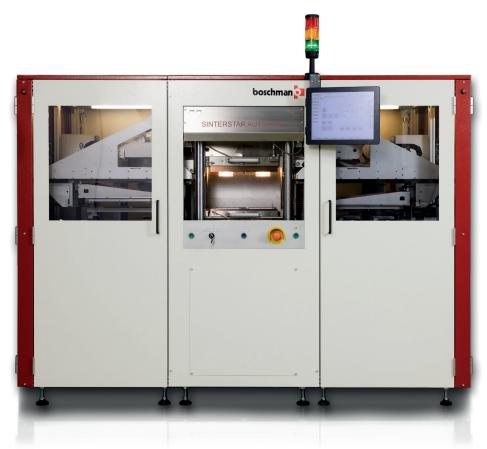
The fully automatic Inline-F-XL-HC can be integrated in the customers automated assembly line. The system is equiped with preheating and cooling stations.
