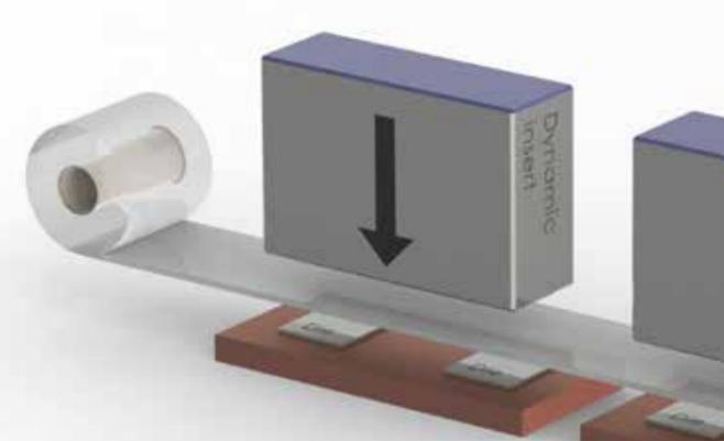
We can use up to 300 um protection tape which also serves to equalize pressure on dies which have a small die height difference.
