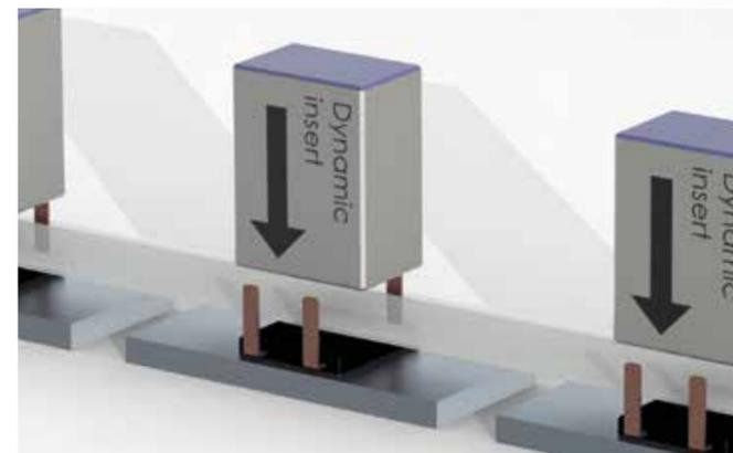
Each insert presses on one individual package with exact pressure control.
