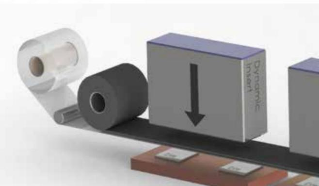
Double film handling. A thick compensation layer can be handled in combination with a protective layer.
