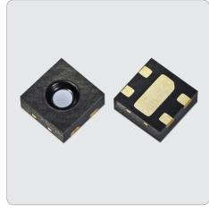
Humidity sensor on lead frame in QFN package. The top side shows an open (exposed) sensor area. The smallest window that can be designed with Film Assisted Molding is approximately  $\emptyset$  0.30 mm.
