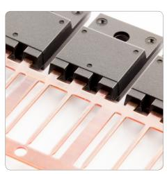
Power package in a TO-3pf/247 layout. This package layout is now also available with single-or double sided Ag-sintering (clip) for optimum thermal performance.
