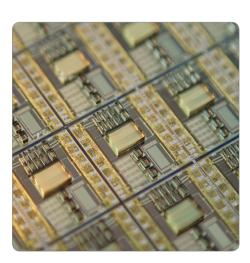
An optical multi-sensor wafer using Through Polymer Via (TPV) technology to create individual optical windows for each detector. This picture shows the wafer before singulation and assembly. Pictures above with courtesy of IC-Haus GmbH and Technical University of Delft.
