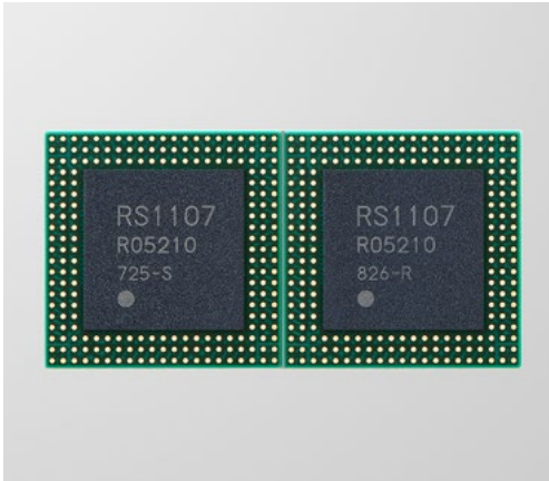
[CONTRAST MARKING] MOULDED PACKAGES (BGA) Vivid colouration that does not engrave the target is possible.
