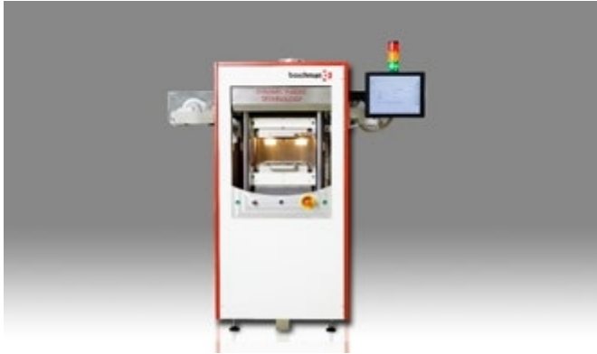
Figure 2: Sinterstar Innovate-F-XL; Universal Sinter System using Film-Assist and Dynamic Insert Technology; Ag Sintering Temperature up to 320 °C; Real time controlled pressure (0.2-40 MPa); Large sintering area 350 x 270 mm; Protecting gas supply optional and Suitable for all kind of carriers, such as: - Lead frames – Substrates - Ceramics – Wafers
