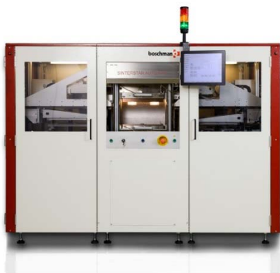
Fig. 4 Boschman Sinterstar Inline F-XL-HC, an advanced industrial sinter press with accurate process control for temperature, pressure and time. The use of dynamic insert technology enables maximum assembly control and verifiable handling.
