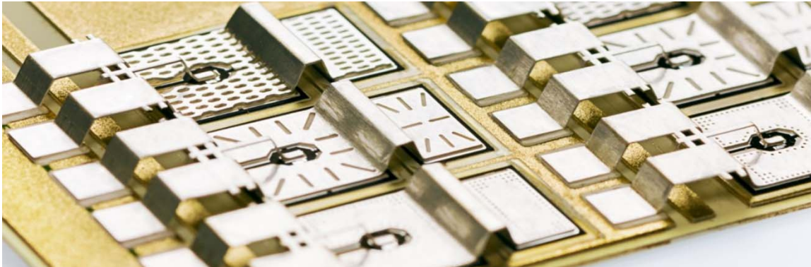
Fig. 5 Several design studies for stress-relieve in clips (Fraunhofer IISB).
