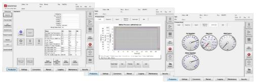
Dashboard with process parameters and real time process graph
